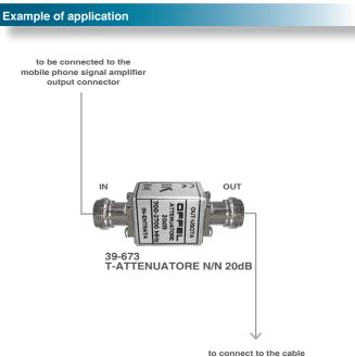
to connect to the cable that goes to the distribution (indoor antenna, splitter, ...)
